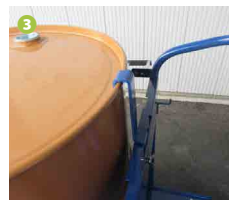
③ Secure the drum with brackets for stable transport.
