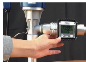
Discharge volume improved to 36 L/min. Auto stop nozzle version maintains stable discharge, delivering 20 L/min.
