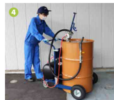
④ Install a power source pump such as an air tank to complete setup.
