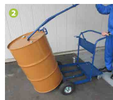
② Place the drum in front of the station trolley and lift it using the handle to slide the base under the drum.
