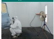
The classic tripod model is designed for stability and less prone to tipping over.
