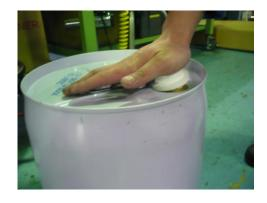
① Lay the adapter on the outlet and press it with your hand.
